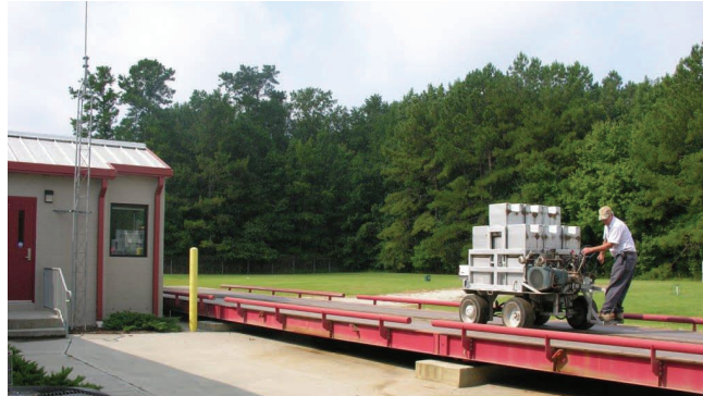
Ken Mallard with Charlotte Scale Company calibrates the scales at the Tuscarora Landfill.
